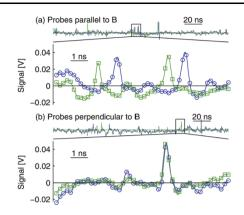
**Fig.13** Observation of phase-space-hole electrostatic structures driven during magnetic reconnection events. a) Propagation between two closely-spaced probes parallel to the magnetic field, b) simultaneous observation on two probes oriented perpendicular to the magnetic field. The time delays combined with known probe separate give the typical size and velocity of the electron holes, which is superthermal compared to the electron temperature. From Fox et al. (2012)
