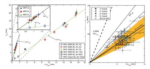
**Fig. 9** (a) Measured half width of the EDR on MRX compared with 2D PIC simulations in Cartesian geometry (Ji et al. 2008) (b) measured half width of the EDR on TREX compared with 2D (solid line) and 3D (orange region) PIC simulations in cylinderical geometry (Greess et al. 2021)
