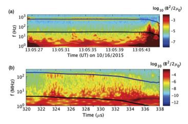
**Fig. 12** Comparison of the whistler wave activity during asymmetric reconnection observed in space (a) and MRX (b). Blue lines indicate half of the local electron cyclotron frequency ( $f_{ce}$ ), while black lines indicate the local lower hybrid frequency ( $f_{LH}$ ). Near the separatrix on the low-density side, whistler waves near 0.5  $f_{ce}$  are observed. After Yoo et al. (2018)
