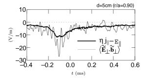
Fig. 11. Time evolution of the measured MHD dynamo electric field  $\langle \widetilde{\mathbf{E}}_{\perp} \cdot \widetilde{\mathbf{B}}_{\perp} \rangle / \overline{B}$  by Langmuir probes [21] in MST, compared with the mismatch  $\eta j_{\parallel} - E_{\parallel}$  in the parallel Ohm's law during a relaxation cycle.
