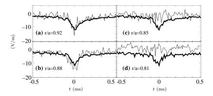
Fig. 12. Time evolution of the measured MHD dynamo electric field  $\langle \widetilde{\mathbf{v}} \times \widetilde{\mathbf{B}} \rangle_{\parallel}$  (light line) by an optical probe [24] in MST, compared with the mismatch  $\eta j_{\parallel} - E_{\parallel}$  (heavy line) in the parallel Ohm's law during a relaxation cycle.
