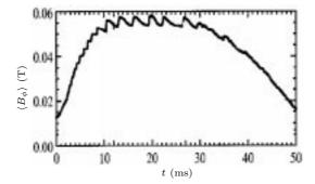
Fig. 8. Toroidal magnetic flux versus time in an RFP experiment.
