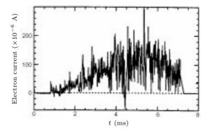
Fig. 14. Evolution of energetic electron current measured by an electrostatic electron energy analyzer with the entrance aligned along the field lineat the edge of an RFP plasma [32].
