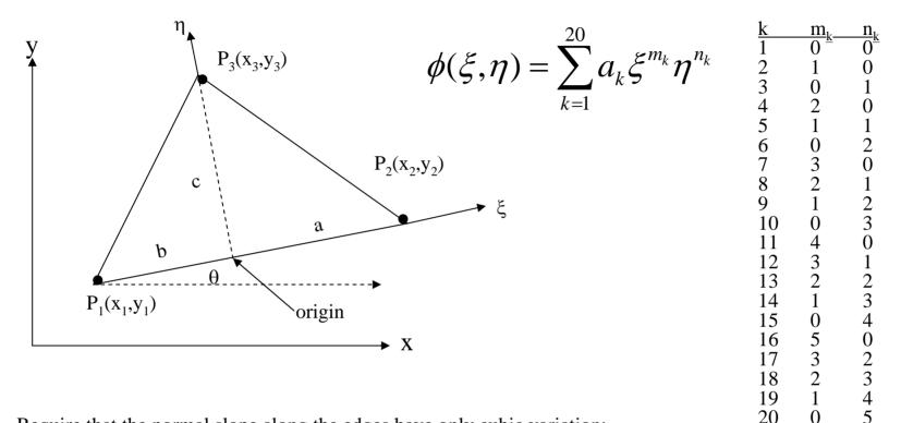
Require that the normal slope along the edges have only cubic variation:  $5b^4ca_{16} + (3b^2c^3 - 2b^4c)a_{17} + (2bc^4 - 3b^3c^2)a_{18} + (c^5 - 4b^2c^3)a_{19} - 5bc^4a_{20} = 0$  $5a^{4}ca_{16} + (3a^{2}c^{3} - 2a^{4}c)a_{17} + (-2ac^{4} - 3a^{3}c^{2})a_{18} + (c^{5} - 4a^{2}c^{3})a_{19} - 5ac^{4}a_{20} = 0$
