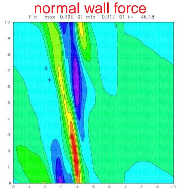
Normal force density at  $t = 46.18\tau_A$ , when it is maximum,  $f_n(\theta/2\pi, \phi/2\pi)$ , where  $\theta$  is the poloidal angle from the origin, and  $\phi$  is the toroidal angle. The horizontal axis is  $\theta/2\pi$ , and the horizontal axis is  $\phi/2\pi$ . The force is concentrated near the top of the wall, on the inboard side.
