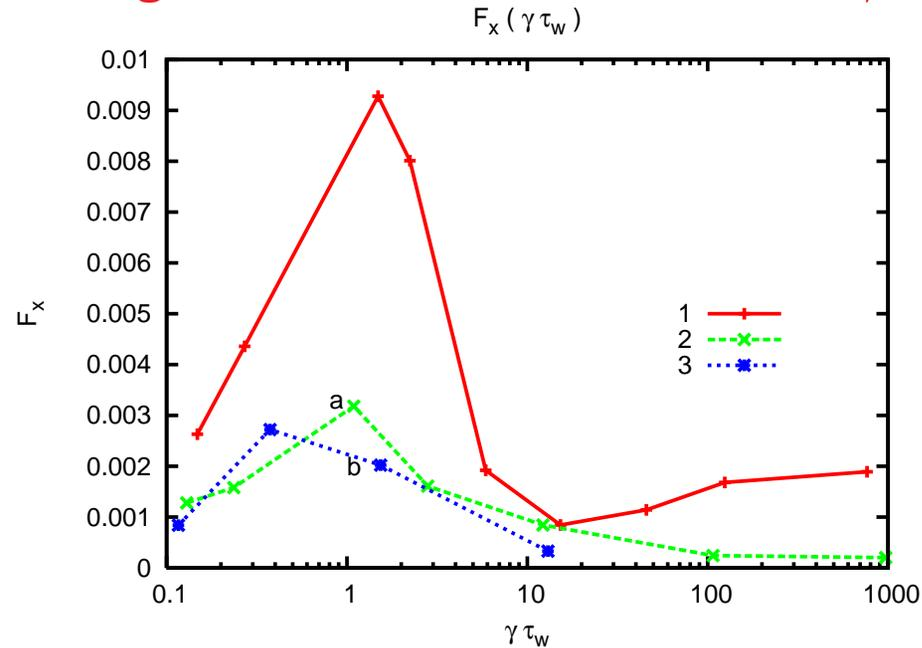
The force tends to a limit for an ideal conducting wall  $\gamma\tau_w \rightarrow \infty$ , and is zero for  $\tau_w = 0$ . The force has a maximum for  $\gamma\tau_w \approx 1$ . The curves correspond to different initial rescaling of the equilibrium: “1” –  $q_0 = .6$ , “2” –  $q_0 = .8$ , “3” –  $q_0 = 1.1$ . The difference between force “1” and “2” is  $\propto \gamma$ .
