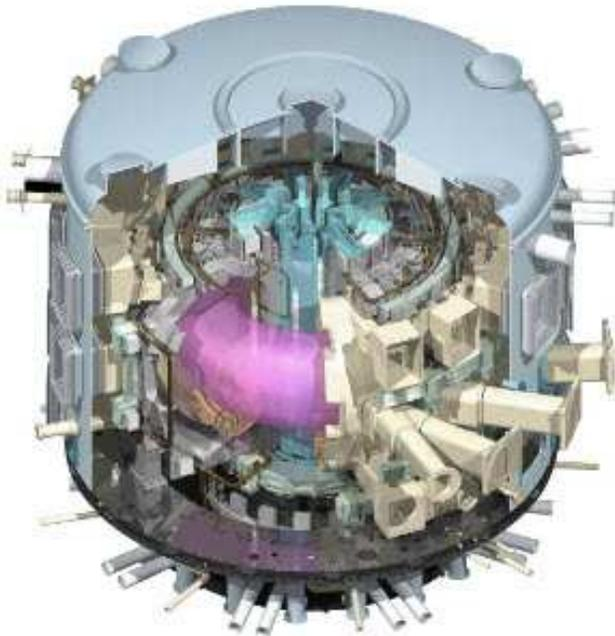
Disruptions in ITER can cause large electromechanical stress on conducting structures. In particular, toroidally asymmetric magnetic perturbations can produce a sideways force. This research is concerned with the sideways force produced by a vertical displacement event (VDE) and a tearing mode or kink mode.
