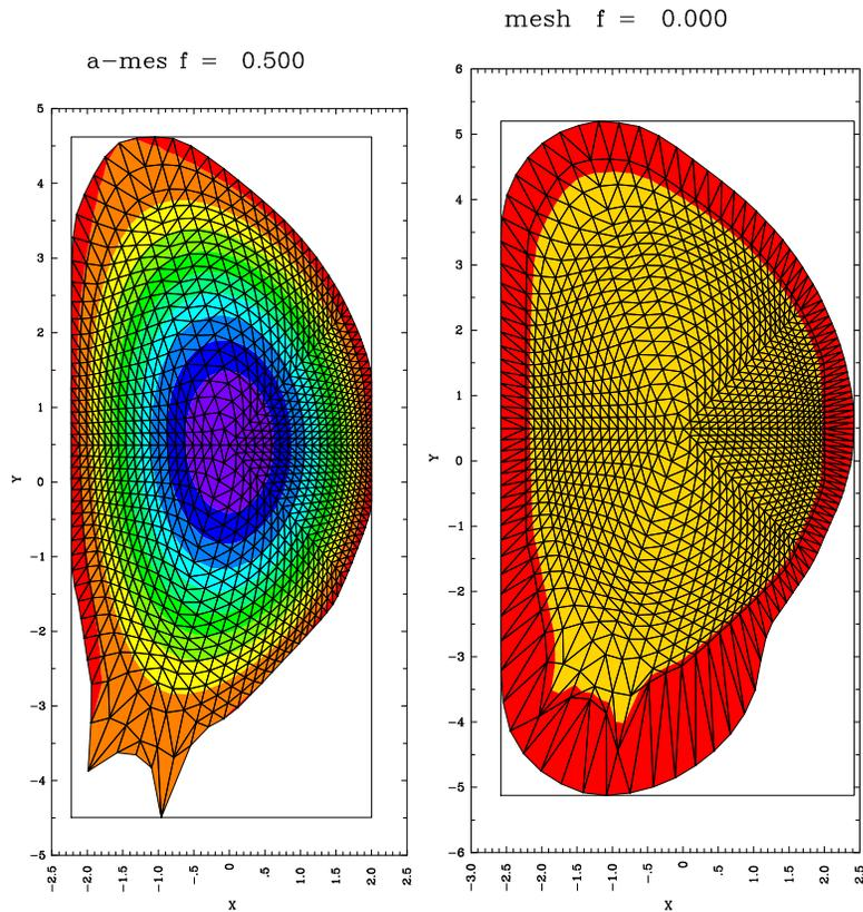
ITER has two walls.  $\tau_w^{outer} \gg \tau_w^{inner}$ . M3D modeling assumes  $\tau_w^{inner} = 0$ . The magnetic field is continuous at inner wall, no force on inner wall. In between is a 3D blanket structure with intermediate penetration time,
