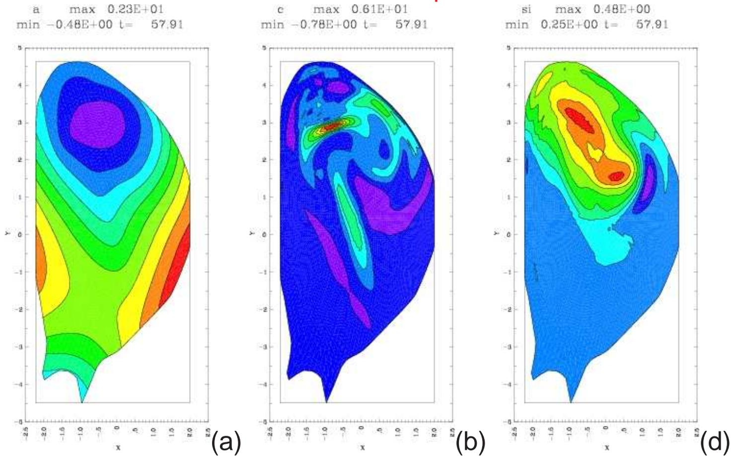
The nonlinear kink mode at time  $t = 57.91\tau_A$ , showing (a) poloidal flux  $\psi$ , (b) toroidal current  $-RJ_\phi$ , (c) toroidal field  $RB_\phi$ , at toroidal angle  $\phi = \pi$ . The current is concentrated at the o and x points of  $\psi$ .
