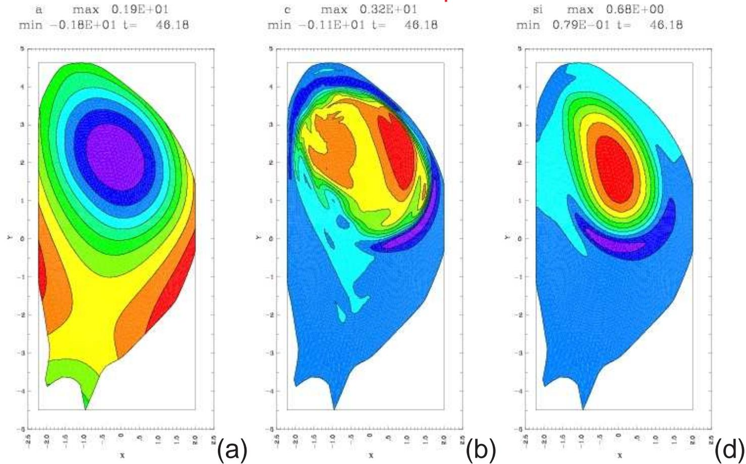
A nonlinear kink mode at time  $t = 46.18\tau_A$ , showing (a) poloidal flux  $\psi$ , (b) toroidal current  $-RJ_\phi$ , (c) toroidal field  $RB_\phi$ , at toroidal angle  $\phi = \pi$ .
