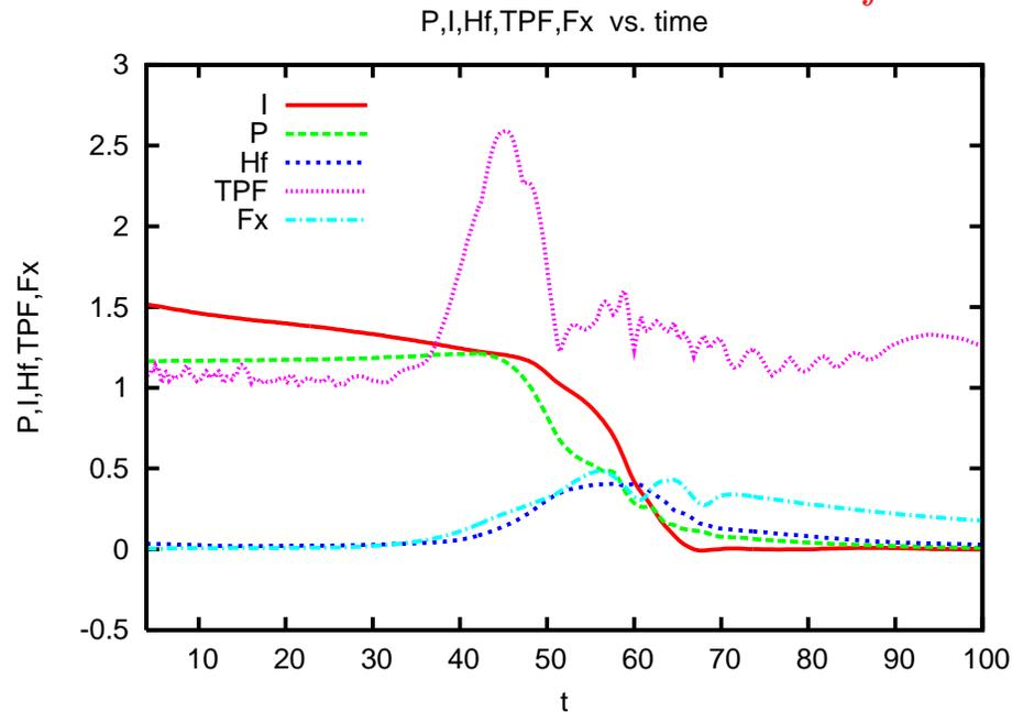
toroidal current  $I$ , pressure  $P$ , TPF, halo current fraction  $H_f$  and horizontal force  $F_x$  as a function of time. The quantities  $I$ ,  $P$ , and  $F_x$  are in arbitrary units. There is a close time correlation of halo current fraction  $H_f$  and horizontal force  $F_x$ .
