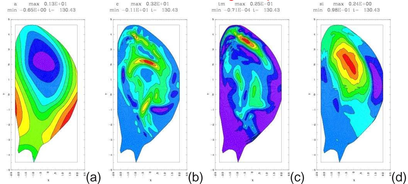
The nonlinear RWM / tearing mode at time  $t = 130.43\tau_A$ , showing (a) poloidal flux  $\psi$ , (b) toroidal current  $-RJ_\phi$ , (c) temperature  $T$ , (d) toroidal field  $RB_\phi$ , at toroidal angle  $\phi = \pi$ . The plasma current and temperature are more broken up, indicating magnetic stochasticity characteristic of “classical” disruptions.
