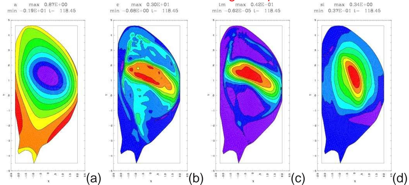
A nonlinear RWM / tearing mode at time  $t = 118.45\tau_A$ , showing (a) poloidal flux  $\psi$ , (b) toroidal current  $-RJ_\phi$ , (c) temperature  $T$ , (d) toroidal field  $RB_\phi$ , at toroidal angle  $\phi = \pi$ . The mode has predominantly  $m, n = 2, 1$  structure.
