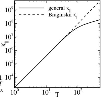
Thermal diffusivity as function of T showing  $T^{5/2}$  response of Braginskii and general closure.
