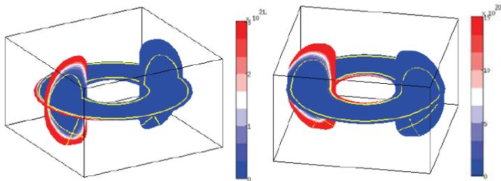
Figure 5. (Left) 3D contour plot of Ne source distribution (Ne density in  $\text{m}^{-3}$ ) for LFS injection with 1/3 toroidal spreading of impurities. (Right) Ne source distribution for HFS injection with 2/3 toroidal spreading of impurities.
