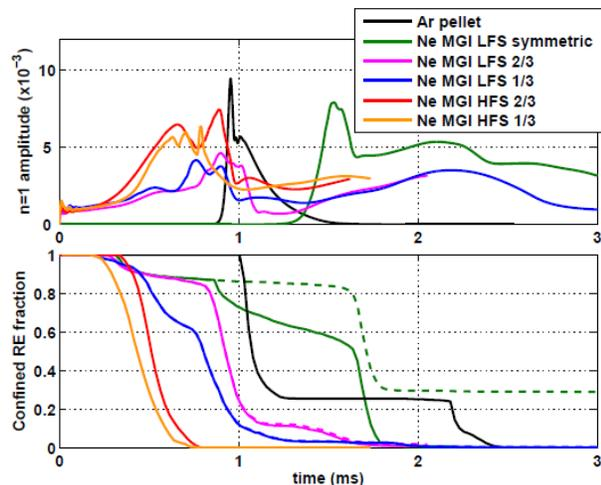
Figure 6. (Top) Amplitude of the  $n=1$  mode for six simulations. (Bottom) Confined fraction of REs versus time for six simulations.
