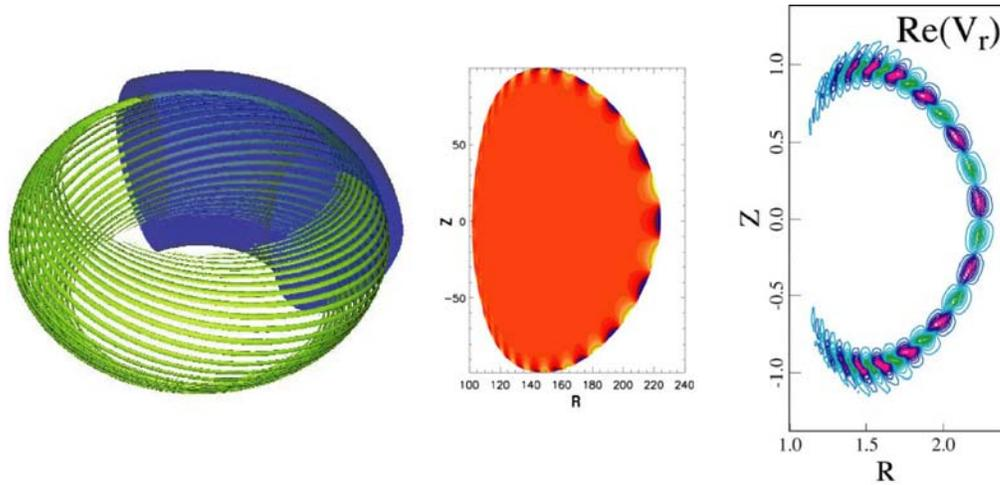
Figure 2. An example of an  $n=21$  eigenfunction (left) and a comparison between the  $n=7$  eigenfunction from ELITE (center) and NIMROD (right), showing the overall agreement in mode structure. The exterior part of the ELITE eigenfunction is not plotted.
