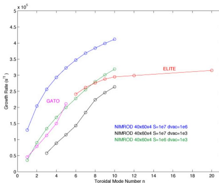
Figure 3. The effects of resistivity changes. Between the blue and black curves the resistivity is only changed in the vacuum region and slightly across the mode region, while viscosity is held fixed.
