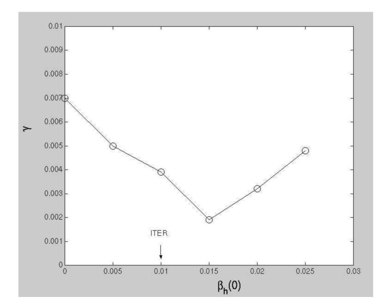
Thermal ion kinetic effects reduce MHD growth rate by half (Kruskal-Oberman)
