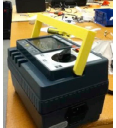
This 3D printed part replaced the meter's original handle. (Photo by Andrew Zwicker)
