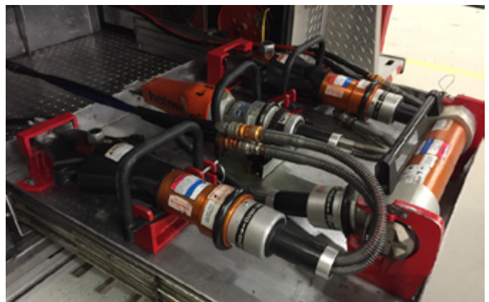
The “Jaws of Life” equipment that lifted the concrete slab. (Photo by Sean Galie)
