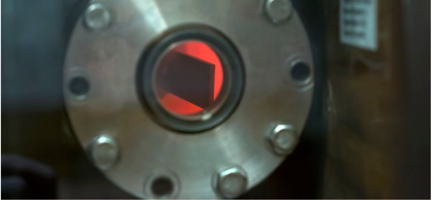
A photo of the titanium coupon being treated in the oxygen plasma.
