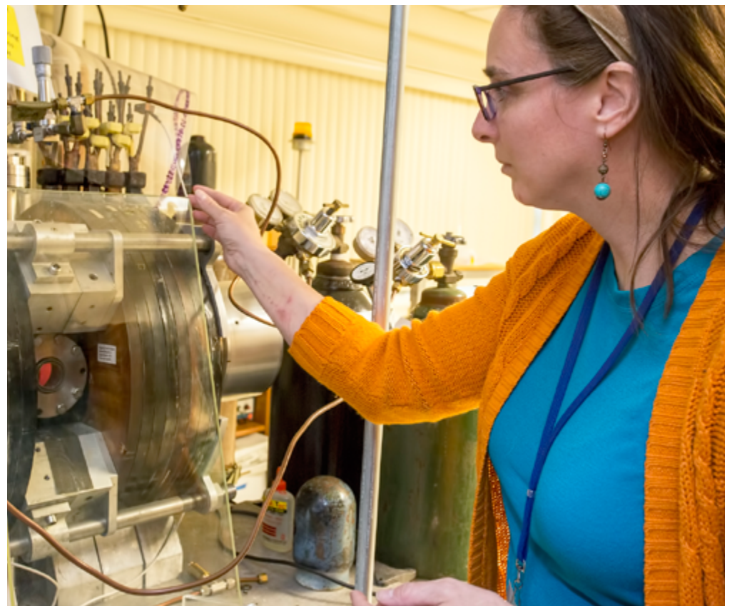
Lenore Rasmussen treats the titanium coupon that holds the gel-like synthetic muscle with an oxygen plasma.
