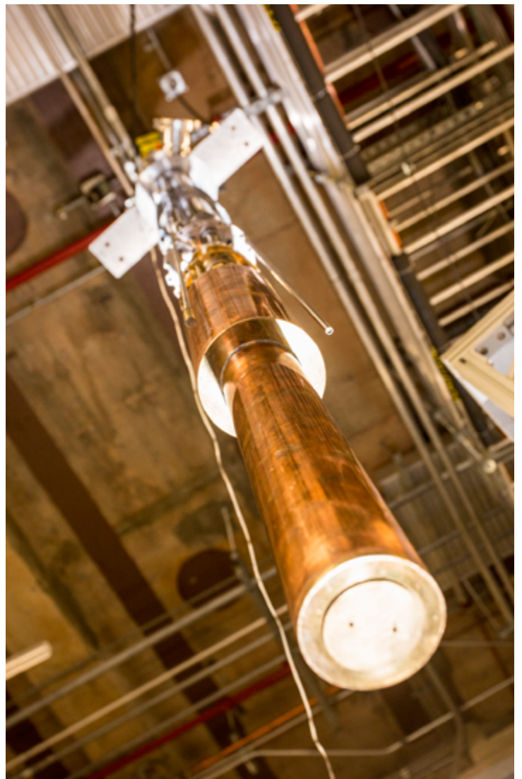
View of the dilution refrigerator that will lower temperature to a small fraction of a degree above absolute zero when connected.
