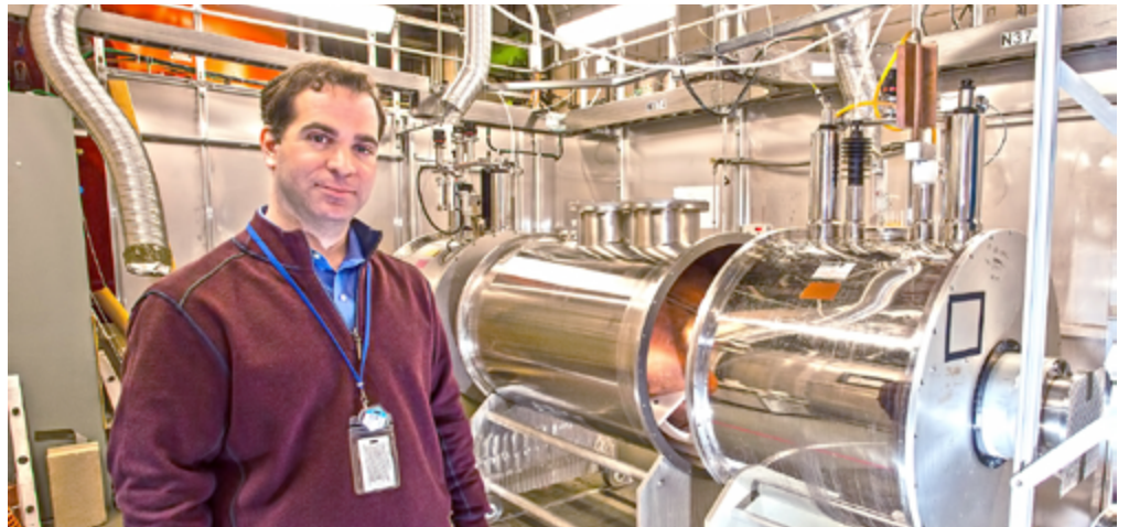
Princeton physicist Chris Tully in the PTOLEMY laboratory. Behind him are powerful superconducting magnets on either side of the vacuum chamber.
