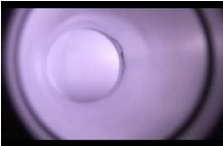
An image of the first plasma in the Stellarator of Costa Rica 1 (SCR-1).
