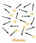
Because of the electric charges carried by electrons and ions, plasma can, in principle, be confined by a magnetic field. In the absence of a magnetic field, the charged particles in plasma move in straight lines and random directions. Since nothing restricts their motion, the charged particles can strike the walls of a containing vessel, thereby cooling the plasma and inhibiting fusion reactions. But in a magnetic field, the particles are forced to follow spiral paths about the field lines.
