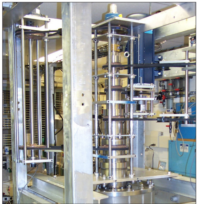
Photo of the MRI apparatus showing the elaborate driving mechanisms for the concentric cylinders.
