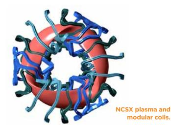
of an inch of design specifications, or about the thickness of a few sheets of paper, in order to maintain the correct shape of the magnetic field. These exacting tolerances ensure that the required magnetic field geometry is achieved with high accuracy.
