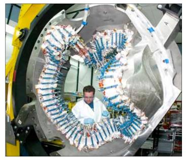
Winding of an NCSX modular field coil.
