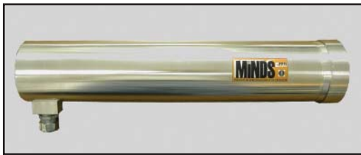
Figure 11. The detectors for PPPL's Miniature Integrated Nuclear Detection System (MINDS) are enclosed in an aluminum case.
