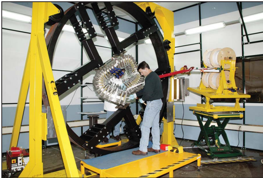
Figure 10. Vertical turning fixture for the winding of National Compact Stellarator Experiment modular field coils.
