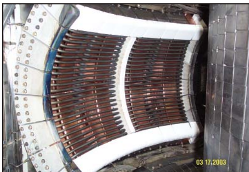
Figure 11. The four-strap ICRF antenna with its former insulating tiles (left) and its new all-metal protection tiles (right).
