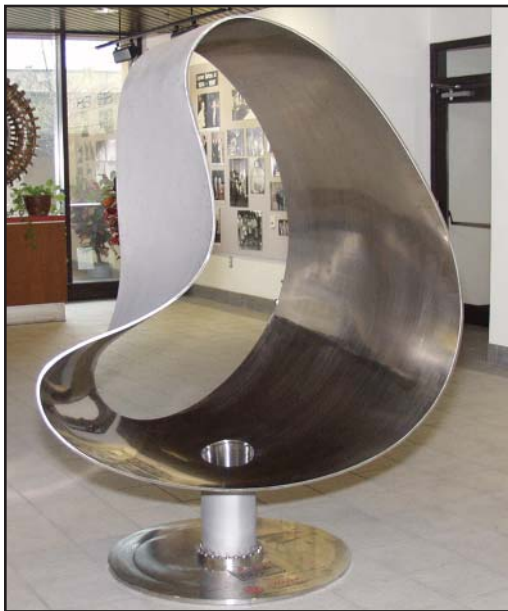
Figure 8. A prototype National Compact Stellarator Experiment vacuum vessel sub-assembly manufactured by Major Tool and Machine, Inc.
