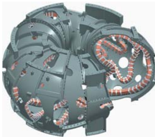
Figure 4. The National Compact Stellarator Experiment modular coils are bolted together to form a shell structure.
