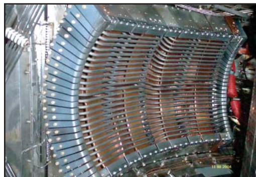
Figure 11. The four-strap ICRF antenna with its former insulating tiles (left) and its new all-metal protection tiles (right).
