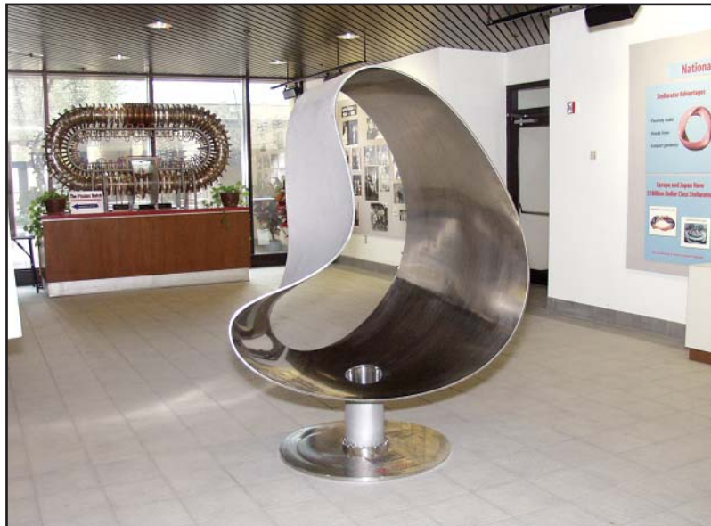
Figure 4. A full-scale 20-degree prototype section of the NCSX vacuum vessel produced by the Major Tool and Machine, Inc., team.
