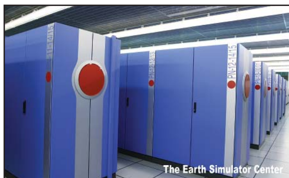
Figure 15. Modern parallel-vector computers: (left) The Cray X1 at the Oak Ridge National Laboratory (ORNL) and (right) the Earth Simulator in Yokohama, Japan. [Photos courtesy of the National Leadership Computing Facility at ORNL and the Earth Simulator Center/JAMSTEC (Copyrighted), respectively.]
