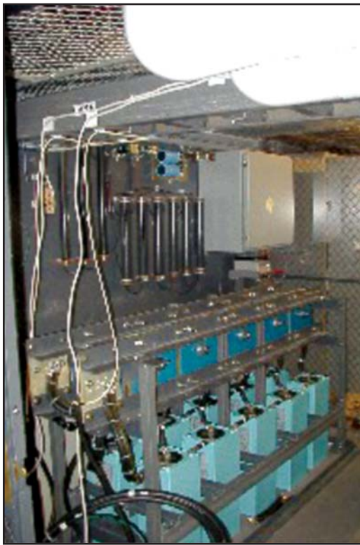
Figure 1. New capacitor bank for coaxial helicity injection start-up experiments on the National Spherical Torus Experiment.
