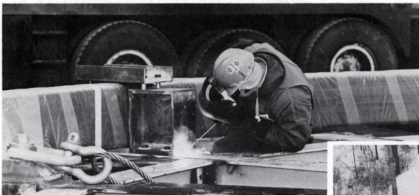
A workman welds support blocks onto the lifting frame holding coil stack number nine. The blocks allow the frame to be tilted while holding the coil securely in place, preventing damage.
