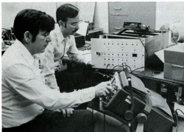
George Renda (left) and Vincent Mastrocola run a calibration check on a bolometer chassis.
