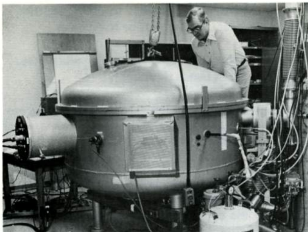
Bill Opperman monitors a vacuum chamber containing a focus coil assembly. The assembly will be part of a windowless ccd being developed for a sounding rocket payload.
