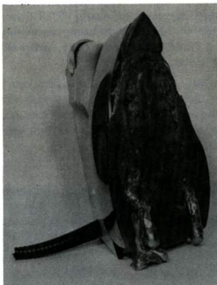
The remains of Jerry Newton's iron reflects the intense heat buildup that resulted in the melting of the iron's aluminum components.
