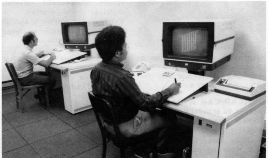
Designers working on the CAD/CAM system can rotate, enlarge, reduce or add color to the three-dimensional images on their workstation monitor screen by entering a simple set of commands.
