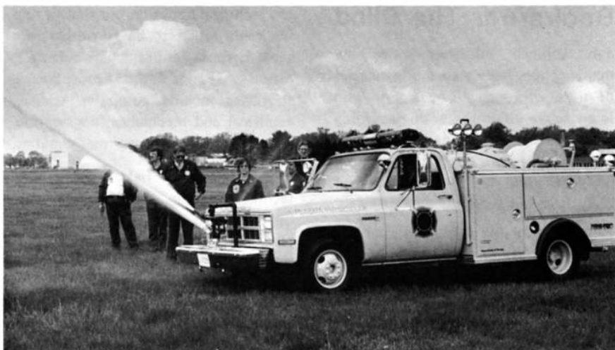
The Emergency Services Unit added a sixth vehicle to its fleet with the acquisition of a Rapid Intervention Vehicle (RIV). The vehicle features front and rear bumper-mounted turrets, which can dispense either foam or dry chemical extinguishing agents, or a combination of both. The front turret is controllable from the cab of the RIV, allowing firefighters to combat fires in areas where on-foot entry might be dangerous. The vehicle also carries approximately 200 feet of fire hose.
