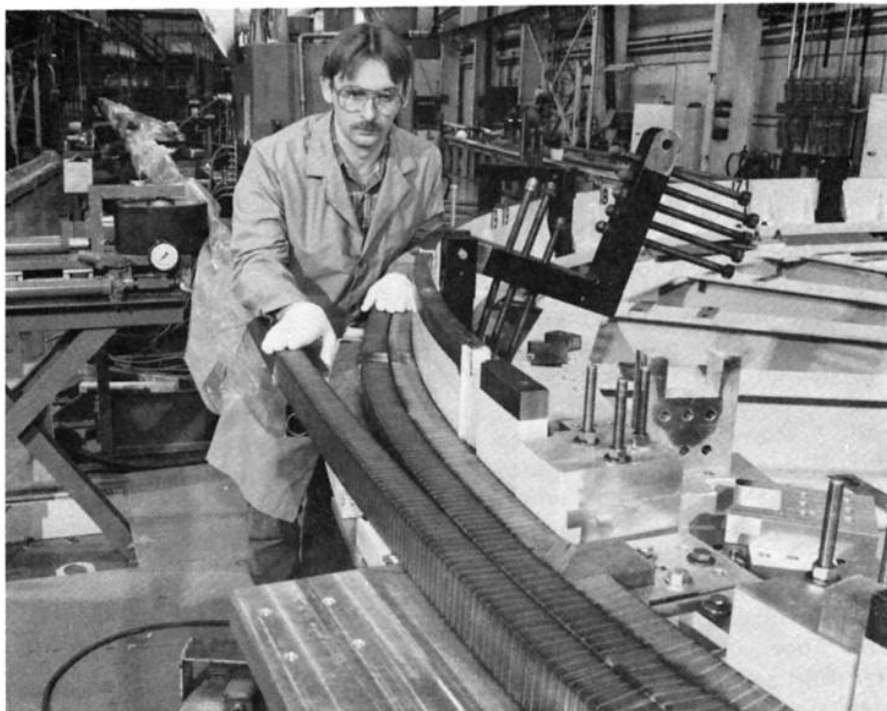
Glenn Northey, lead ATF technician, monitors the winding of one of the main VF coils.
