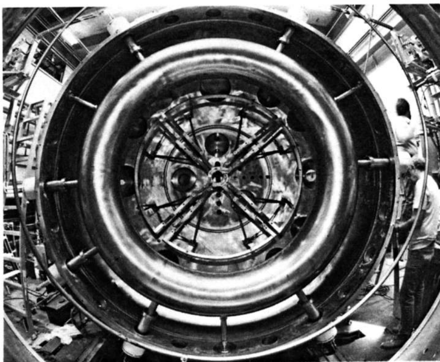
The passive figure-8 coil stabilization system is visible through the newly installed S-1 flux core
