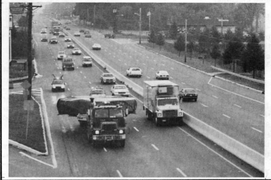
The first of the vertical field coils PPL's Coil Shop wound for the Advanced Toroidal Facility (ATF) at Oak Ridge National Laboratory hit the road September 5. Traveling by truck to Oak Ridge were two outer coil assemblies, an inner coil assembly and its support structure, and a lifting fixture, constituting 63,000 pounds of coil and structure. The coils will be stored at Oak Ridge until ATF assembly begins this fall.
