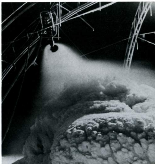
A nighttime shot of the snowmaker in operation. The dome, not present in the photo, is supported by the curved members.
