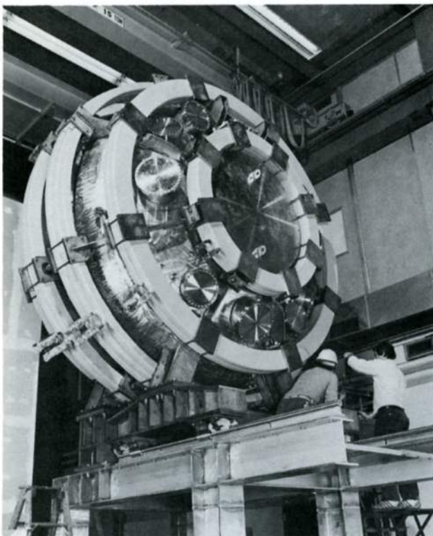
Testing continues on the Spheromak, which has been mounted on its stand. The machine is due to receive its flux core in August.
