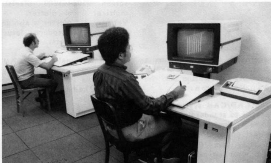
Designers working on the CAD/CAM system can rotate, enlarge, reduce or add color to the three-dimensional images on their workstation monitor screen by entering a simple set of commands.
