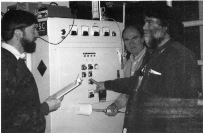
A radio frequency oven from the U.S. Department of Agriculture (USDA) is presently at PPPL for testing and modifications as part of a collaborative project between PPPL and the USDA to develop new pasteurization methods that use radio frequency (RF) waves and microwave heating. Next to the oven are members of the PPPL team, including (from left), Chris Brunkhorst, Elmer Fredd, and Dave Ciotti. Not pictured is Randy Wilson. The machine is expected to be returned to the USDA's Eastern Regional Research Center in Philadelphia sometime this summer, where the pasteurization experiments will take place.
