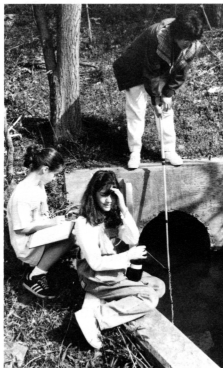
PPPL's Virginia Finley holds a flow meter probe in the basin discharge while Jill Mansfield (left), daughter of Dennis Mansfield, and Ashley Taylor (middle), daughter of Jim Taylor, read and record flow for how many gallons per minute were being discharged. Later, the three calculated that a total of 429,800 gallons would flow from the basin on that day and then saved this data on Finley's spreadsheet, which is used to report flow to the Department of Environmental Protection each month.
