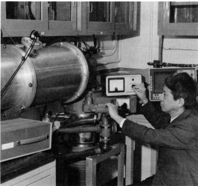
Hideo Okuda measures the pressure of the vacuum tank using a discharge vacuum gauge.
