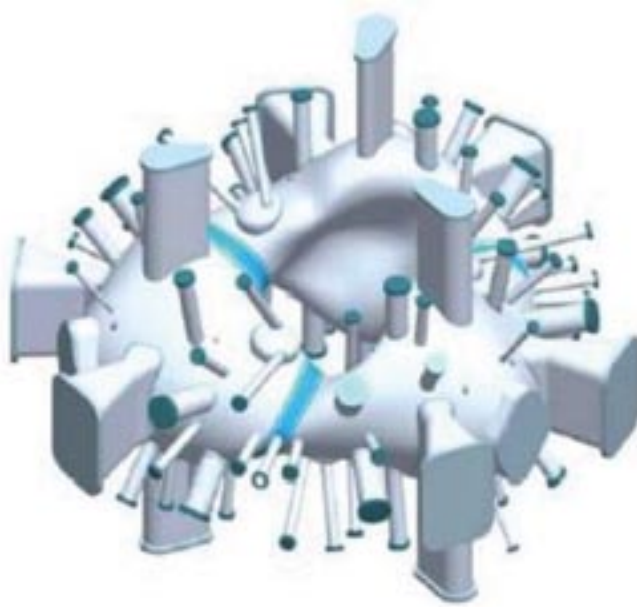
The NCSX vacuum vessel.
