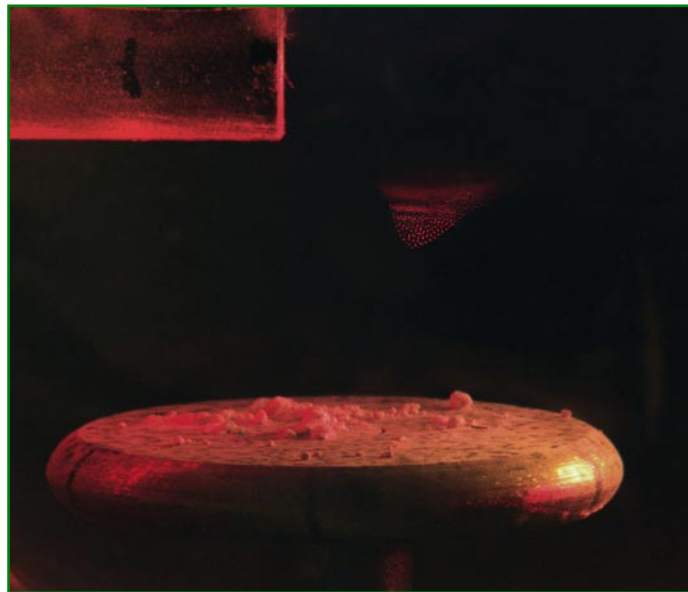
“Plasma Table,” by PPPL’s Elle Starkman and Andrew Post-Zwicker, won first place in the “Art of Science” contest. The image features a dust cloud of silica microspheres suspended in a plasma and illuminated by laser light.
