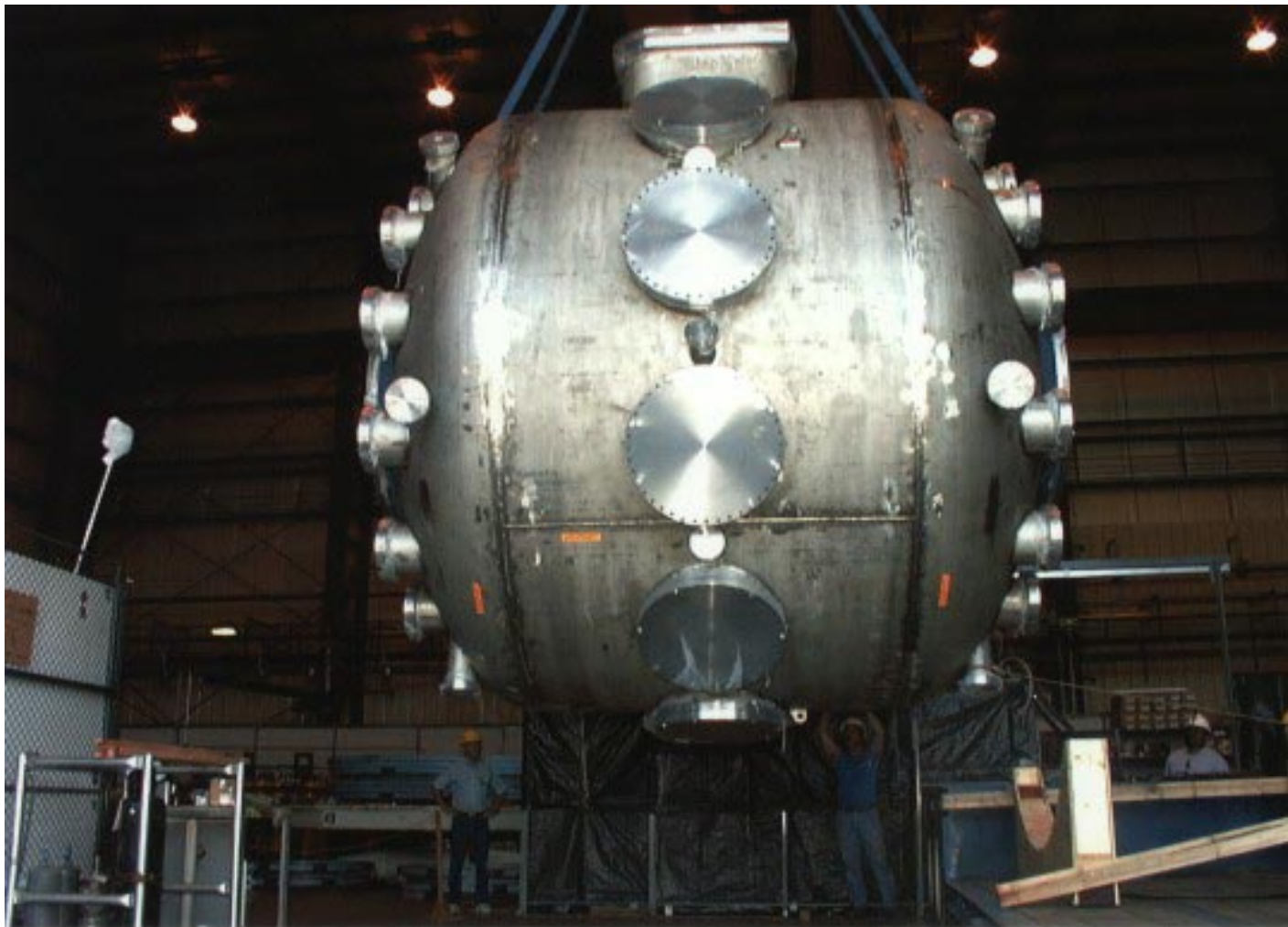
The 23,000-pound vacuum vessel for the National Spherical Torus Experiment arrived at the Lab on August 5. The arrival marks a major step in the construction of the new device.
