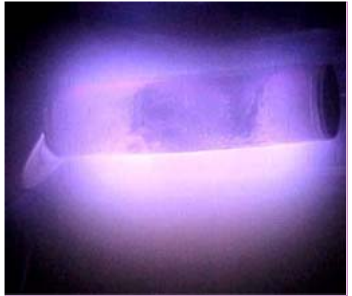
Above is the head in the CDX-U vacuum chamber during argon glow-discharge cleaning. The center of the head, where the interaction with the plasma was the strongest, still shows a coating. The surface near each end is cleaner. The previously bare region toward the right of the head has become “wetted” with lithium.
