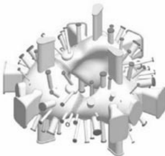
The NCSX vacuum vessel.
