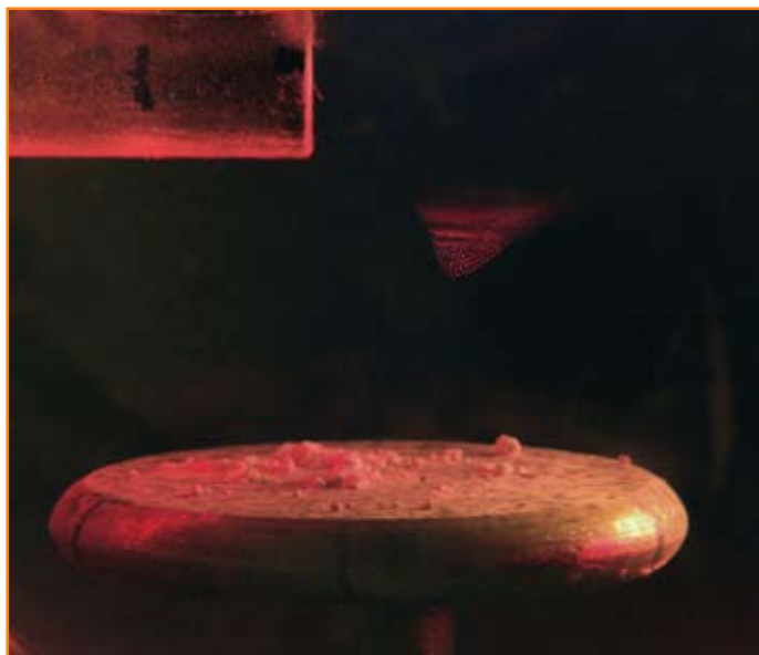
Above, Andrew Post-Zwicker (left) and Elle Starkman with their collaborative art, "Plasma Table." At right is the first-place winning photo, which features a dust cloud of silica microspheres suspended in a plasma and illuminated by laser light.
