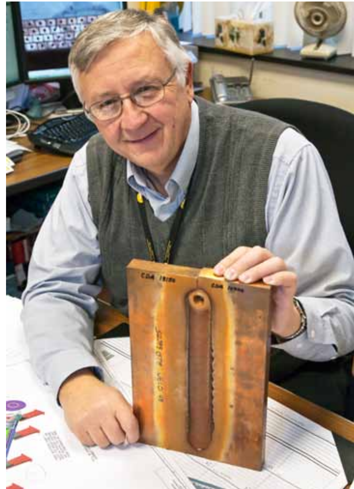
James Chrzanowski displays the seamless bond that friction stir welding created between two dissimilar types of copper plate.
