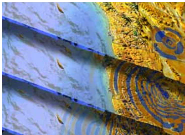
Spectral-element simulation of earthquake dynamics. The sequence of three snapshots depicted here illustrates wave propagation in southern California.
