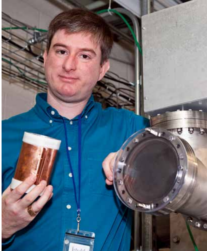
Erik Gilson with a copper-clad plasma source module and chamber for testing the units.
