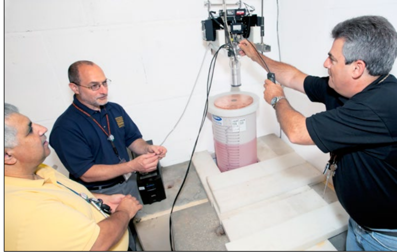
George Ascione, far right, positions gamma ray detector over copper plate and a coupon of molybdenum.
