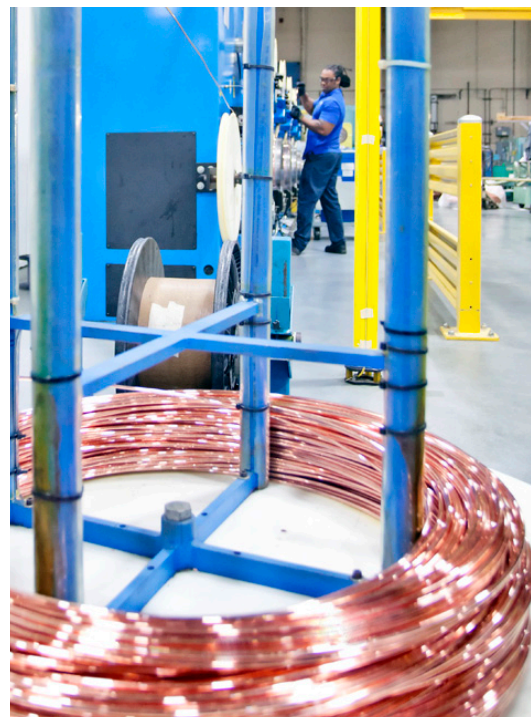
This superconducting wire will become thin as a needle when Oxford Superconducting Technology finishes manufacturing it. (Photo credit: Elle Starkman, PPPL Office Of Communications)
