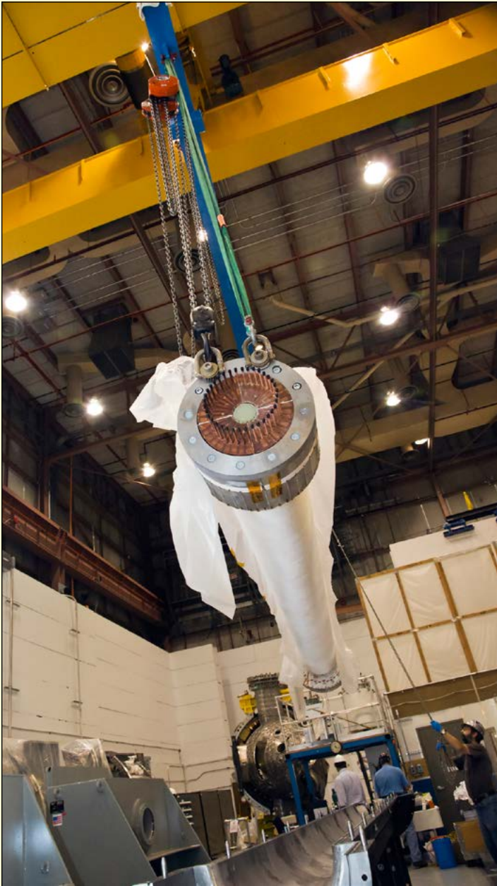
Technicians prepare to lower the taped bundle of coils into the mold.
