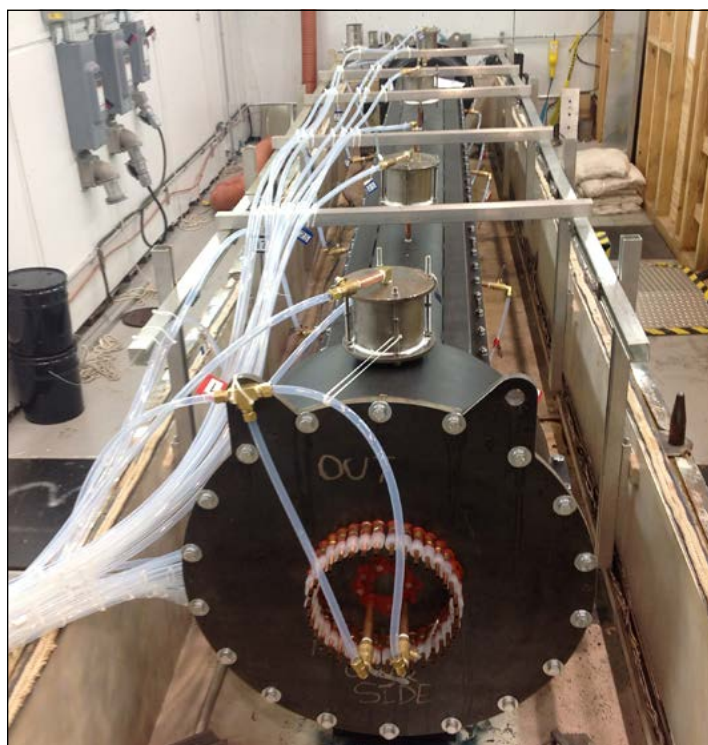
The full bundle of conductors inside the mold. (Photo by Jim Chrzanowski).
