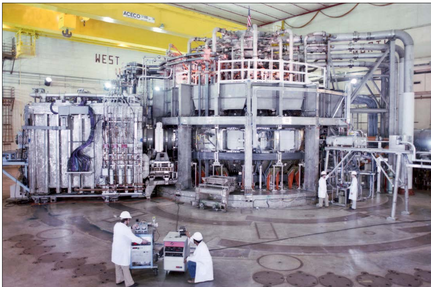
The Tokamak Fusion Test Reactor (TFTR) set then-world records by producing 9.2 million watts of fusion power in 1994 and reaching a plasma temperature of 510 million degrees Celsius in 1995 before being decommissioned later in the decade.
