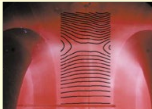
Magnetic reconnection seen in MRX: Oppositely directed field lines (measured) merge and reconnect.
