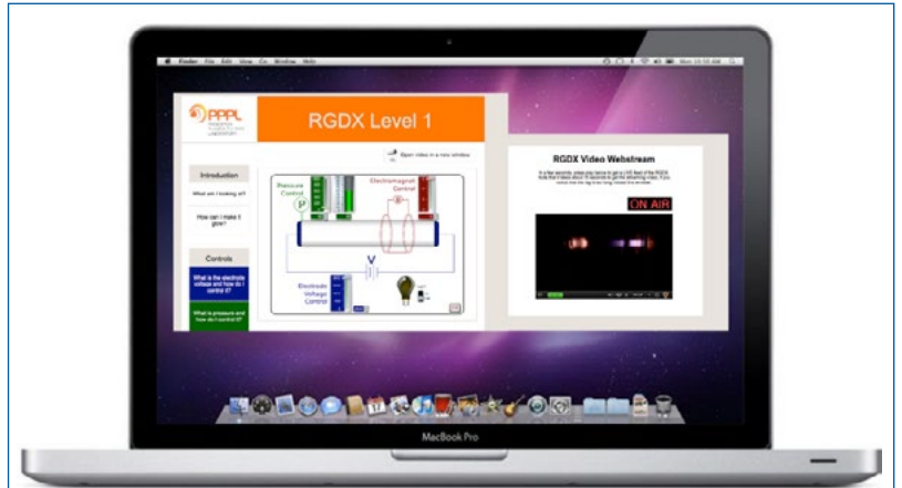
The user can operate the experiment with a set of controls, shown on the left side of the screen, and watch the effect on the apparatus at PPPL using the webstream video, shown on the right.
