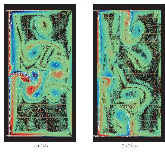
Figure 4. Instantaneous contours of azimuthal vorticity and vector field of poloidal velocity for Re = 6200 in the case of lids (a) and rings (b). The EC and outward radial jet near the midplane in the case of lids are severly disrupted in the setup with rings due to alternating inward—outward Ekman flows.
