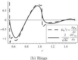
**Figure 2.** Steady-state scaled radial wall shear (——) and near-wall net radial force (---) for Re = 620 in the case of lids (a) and rings (b). The definite negative net radial force in the lids case (a) results in the inward radial Ekman flow with negative radial wall shear being disrupted in the case of rings (b) by the alternating sign of the net radial force that correlates well with the sign of the wall shear and thus with the alternating directions of Ekman flows.
