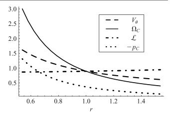
**Figure 1.** The CCF azimuthal velocity  $V_{\theta}$  (---), angular velocity  $\Omega_{\rm C}$  (---), axial angular momentum  $\mathcal{L}=rV_{\theta}$  (----) and minus pressure  $P_{\rm C}$  (----) versus radius. Note the monotonically increasing angular momentum and decreasing angular velocity with radius for centrifugally stable CCF where the 'centrifugal' rotation balances the centripetal pressure gradient leading to zero radial and axial velocities.
