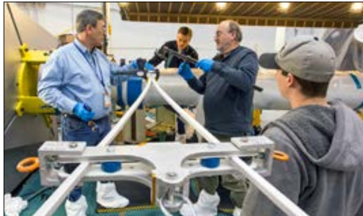
Technicians apply clamps to the insulated conductors before guiding them onto the stack where they are wound tightly by the winding device at the far left. From left to right: technician Andy Carpe; Mike Anderson, senior lead in charge of the coil winding; technicians Dave Moser and Steve Bartzak.
