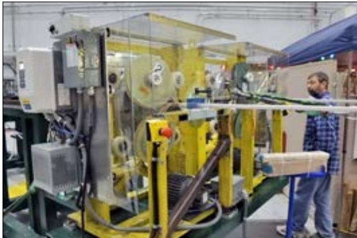
Technician Buddy Kearns examines the tape machines that apply insulation to the copper conductors.
