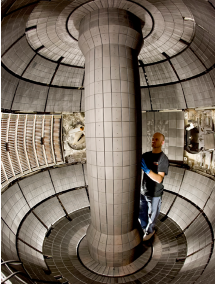
Interior of the NSTX-U showing the completed center stack.
