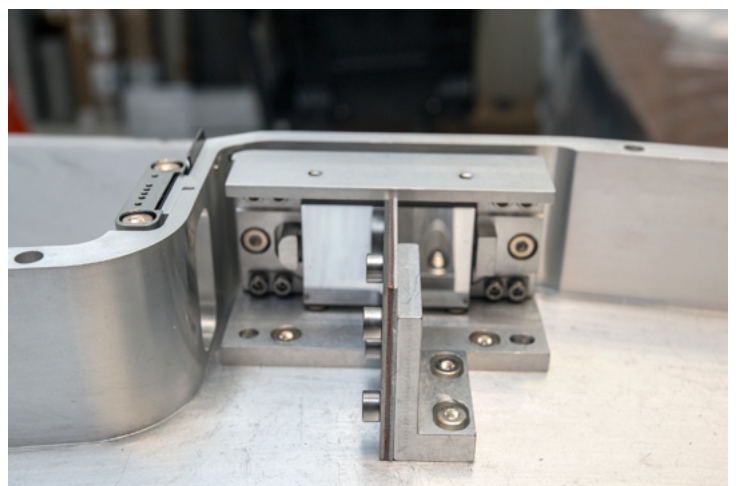
Zoom-in view of the Qz channel. There is a window next to the crystal assembly for allowing X-rays to propagate through and impinge onto the crystal. In front of the crystal is a shielding piece to block scattered X-rays. (Photo by Elle Starkman)
