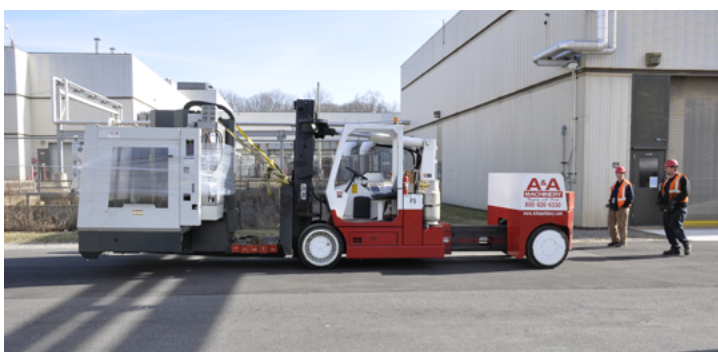
A contractor uses a remote control to operate a forklift carrying a 12,000-pound CNC milling center to the MG Building. (Photo by Ken Bauer)
