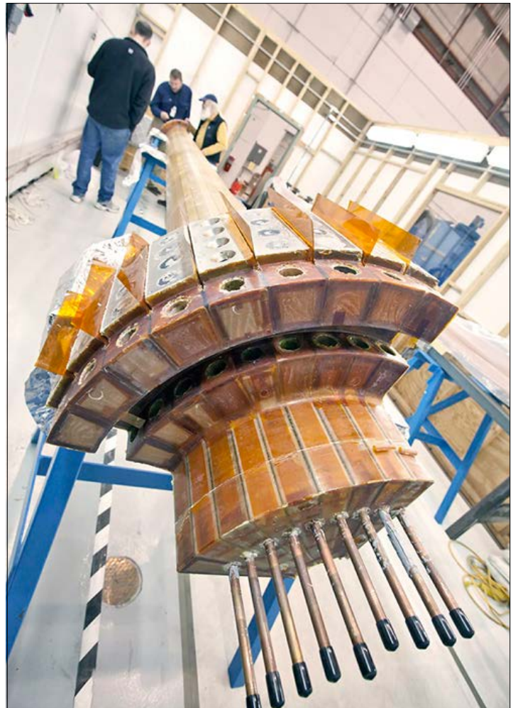
Mission accomplished: The successful procedure capped months of demanding preparations and close teamwork. The cooling tubes in the foreground were soldered along the length of each conductor.
