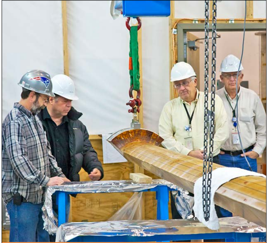
Fresh from the VPI mold: The pressurized treatment produced a uniform application of insulation that showed 20 times more electrical resistance when tested than the minimum amount required.
