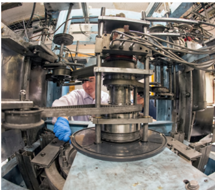
PPPL physicist Erik Gilson and PPPL technician Peter Sloboda make final adjustments to the lid that holds the liquid metal before spinning up the Magnetorotational Instability experiment. (Photo by Elle Starkman)
