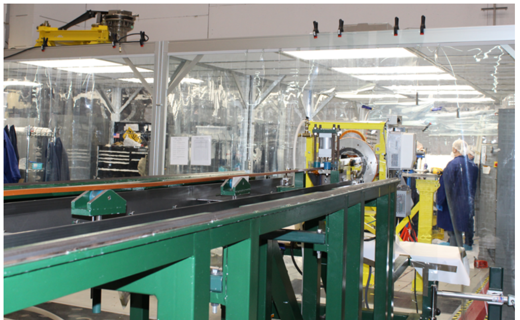
Copper is fed into a coil winding machine where it will later be wound onto a mandrel. (Photo by Jeanne Jackson DeVoe)
