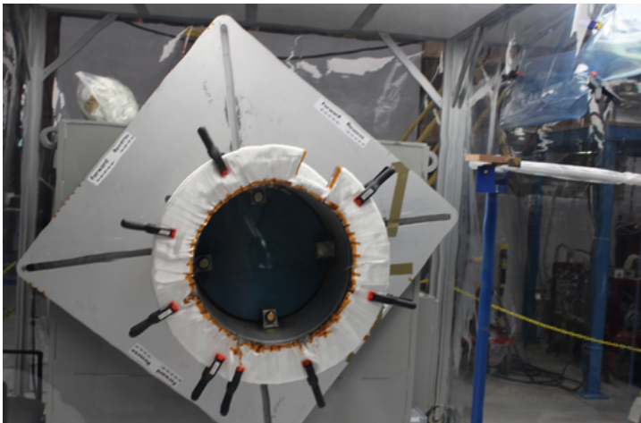
The mandrel onto which the coil will be wound. (Photo by Jeanne Jackson DeVoe)
