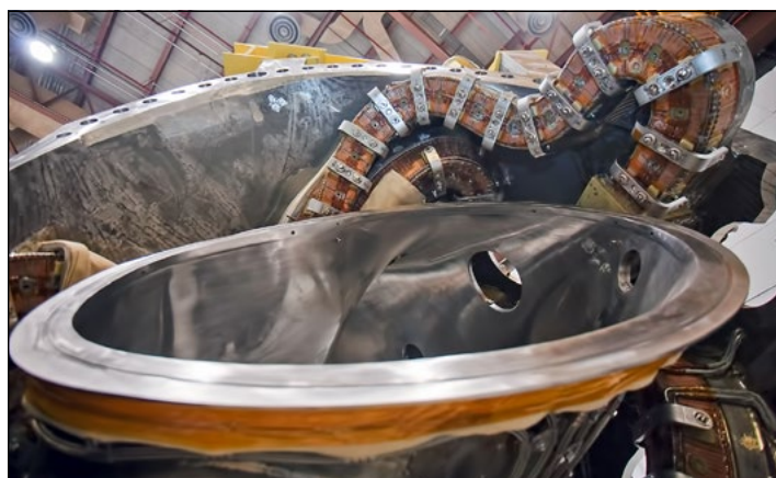
A close-up view of part of a QUASAR coil and vacuum vessel.
