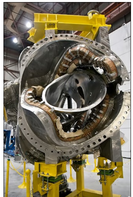
Part of a QUASAR coil and vacuum vessel.
